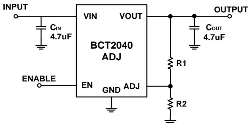
NOTE:  $V_{OUT} = (R1 + R2) / R2 \times 0.8 V$
